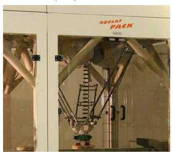
machine completely built by Robertpack, comprising 2x FANUC M3iA/6S robots for the box loading, underbox erector, tray edge closer and a lid setter. At the end of the line, a standalone FANUC M-710iC/70 robot palletizes the boxes. The BRC, IFS, Skal and HACCP certified company complies with the highest quality standards in the industry.
